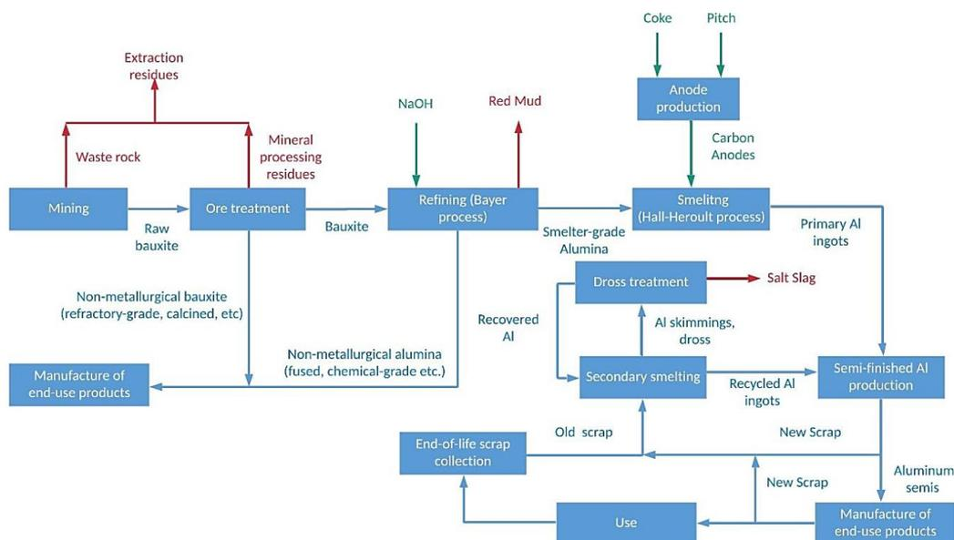
**Figure 1. Simplified flow chart for the entire production of aluminium, with waste streams represented by the red arrows (Georgitakis et al., 2021).**
