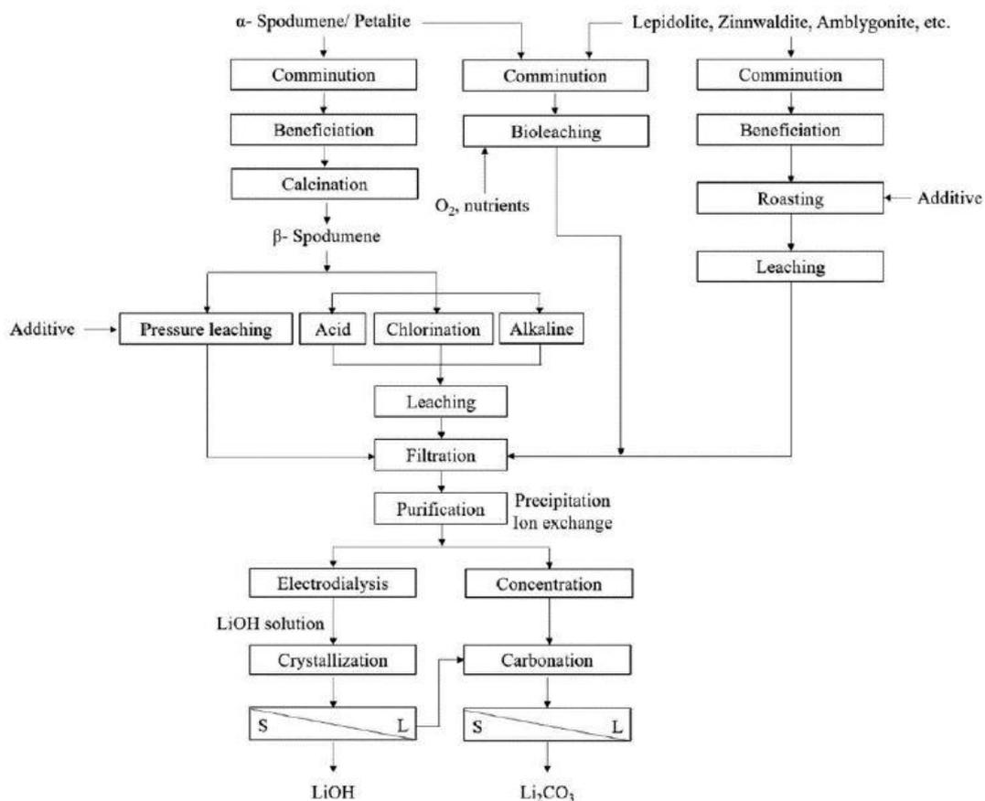
**Figure 25. General steps to produce lithium carbonate and lithium hydroxide from mineral ores and clays. Source: (Meng et al., 2019)**
