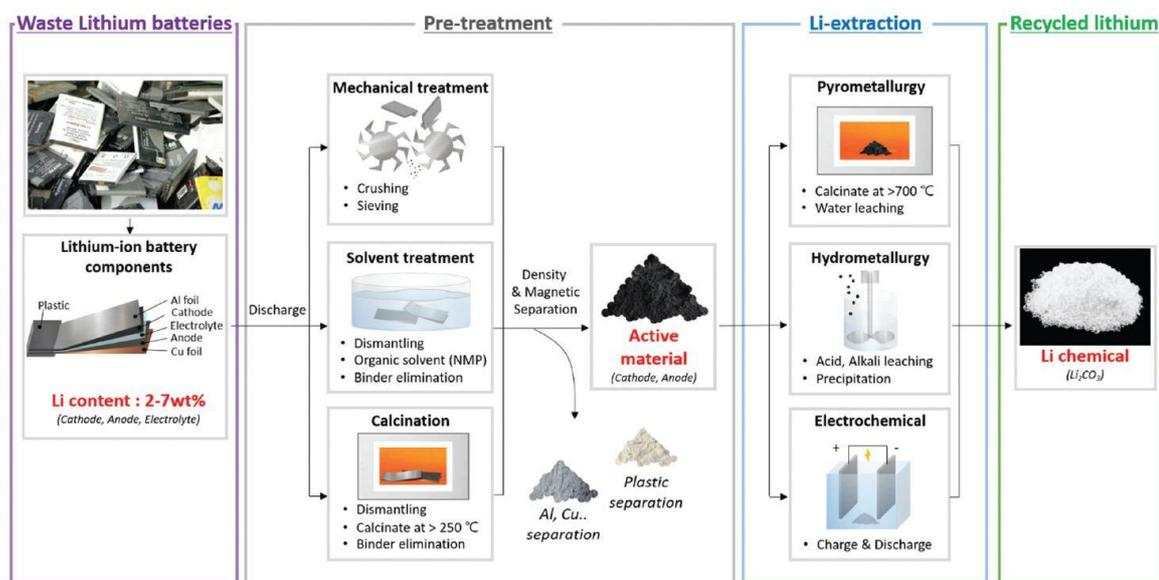
Figure 26. Schematic diagram of the lithium recycling stages and methods from lithium-ion batteries. Source: (Bae and Kim, 2021)
