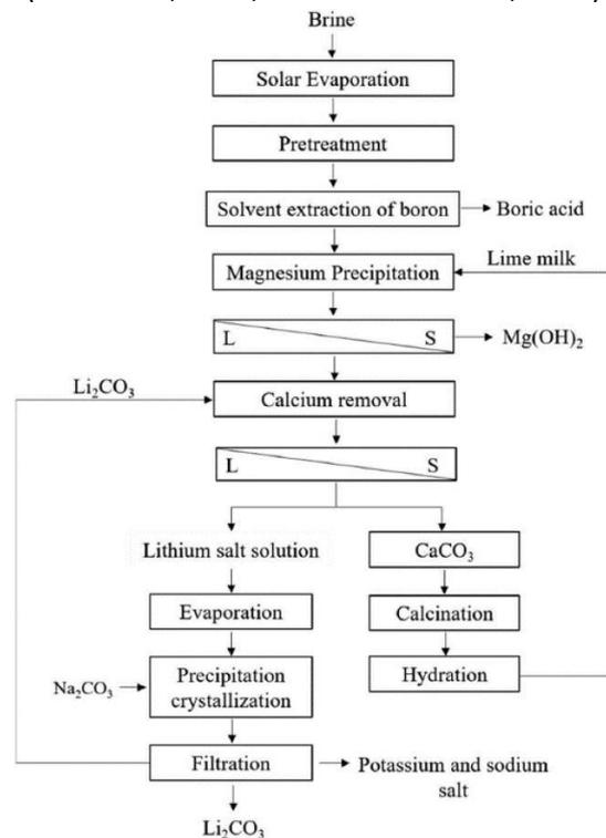
Figure 24. General steps for the production of lithium carbonate from continental brines. Source: (Meng et al., 2019)
